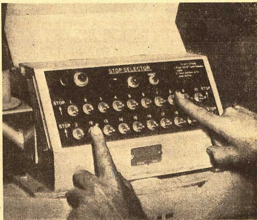
The control board by which the train's journey is preset.
