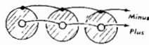
Figure 5. By connecting cells in parallel, the terminal voltage is unaltered but the current handling capacity is multiplied.
