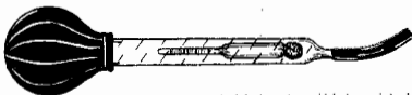
Figure 8. A typical hydrometer, which is used to indicate the condition of accumulator cells.
