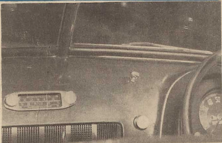
One of the most popular installations—in a Holden. A cut-out is provided in the dash (normally covered by a dress plate) and the set mounts conveniently behind it. The speaker is behind the grill just below the dial, mounted on a simple baffle. The set and power supply are bolted to a bracket which then fastens to the bulkhead. Slots in the underside of the cases allow exact positioning of the units. The front plate may be left off the set, and the dial supported with wooden blocks screwed to the inside edges of the case.
