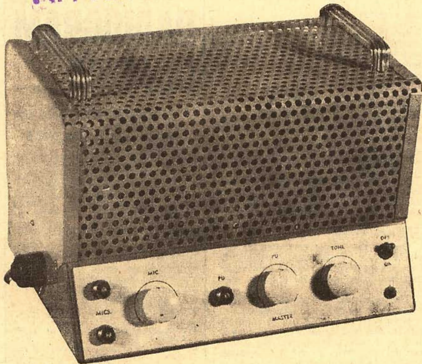
A view of the completed amplifier. Controls from left to right are, two microphone input sockets, the microphone channel volume control, the pickup input socket, the combined pickup volume control and master control for the mixer unit, the tone control, and the on-off switch and indicator bezel.
