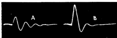
Fig. 5 — Shock tests show effect of magnet. (A) A 10-inch loudspeaker unit with a 10,000-gauss magnet. (B) Same as for part A but with a 14,000-gauss magnet.
