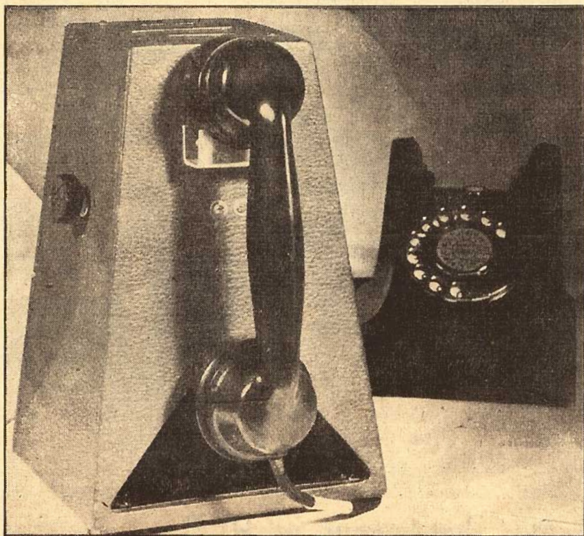
The transistorized telephone amplifier in use. Headpiece is held close to magnetic pickup coil, the output of which is amplified and fed to the speaker mounted in top of case. Volume control is at the side. The horn at the bottom of the case helps to reinforce outgoing speech.
